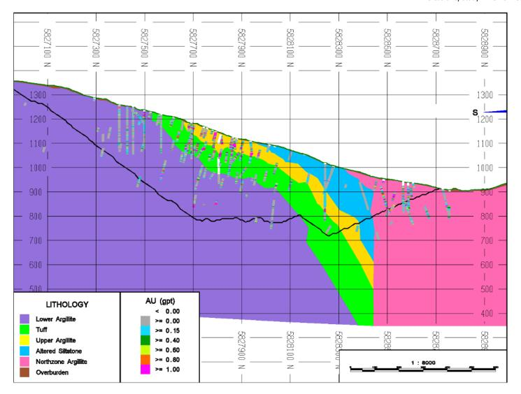
Figure 10-16 Section East 604385 looking West with Drill Grades (+/- 10 m from section) Relative to lithology and Resource Pit Shell
