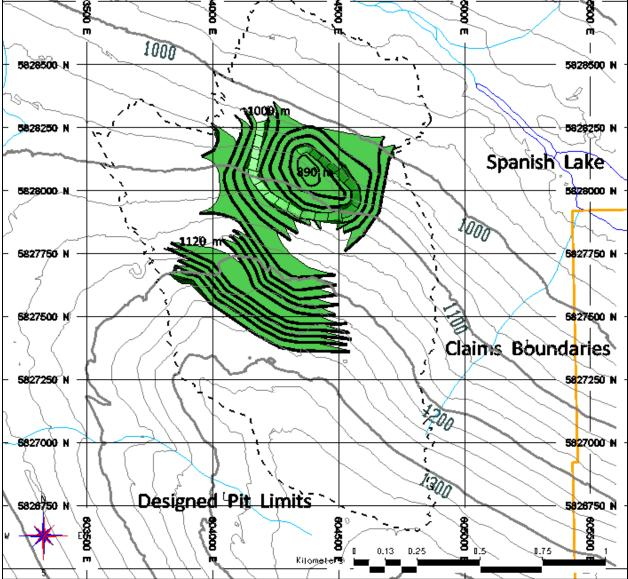
P6228 pushes the central portion of the pit out to the south, mining from the pushback crest at 1220 m elevation down to the pit exit at the 1000 m elevation via external roads: then down the counterclockwise ramp to the pit bottom at the 890 m elevation. This phases development assumes that the preceding phases have mined the benches above the 1220 m elevation.
