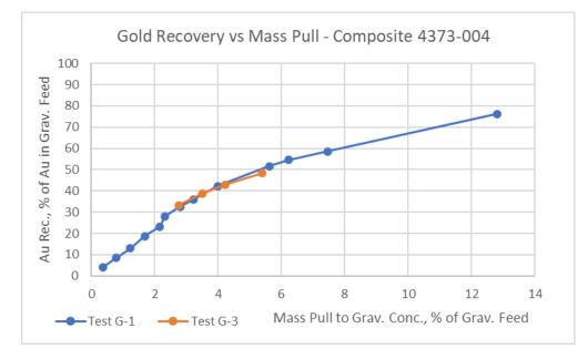
Figure 13-9 Gold Recovery vs Mass Pull, Gravity Concentration, Combined Flotation, Cleaner Tailings, Composite 4373-004, 80%-180µm Feed Size
