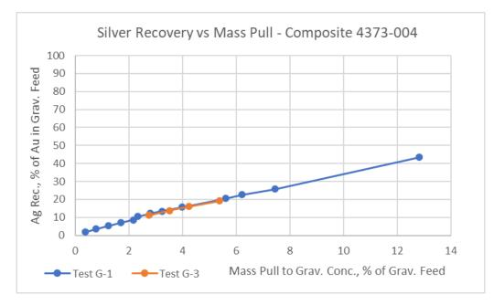
Figure 13-10 Silver Recovery vs. Mass Pull, Gravity Concentration, Combined Flotation, Cleaner Tailings, Composite 4373-004, 80%-180um Feed Size
