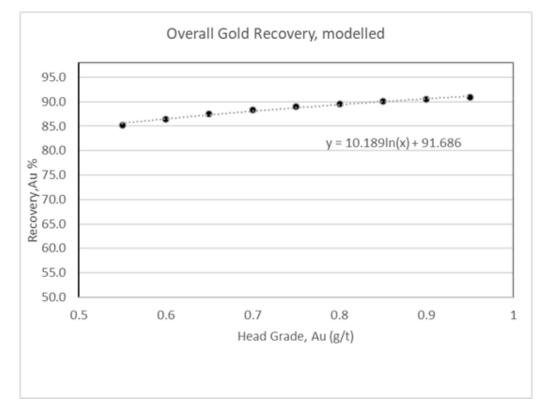
Figure 13-18 Overall Gold Recovery as a Function of Head Grade
