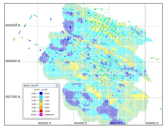
Figure 14-13 Silver Block Grade Estimates and Drillhole Grades – Level 925 El
