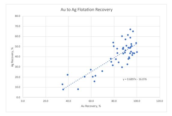
Figure 13-13 Relationship of Gold and Silver Flotation Recovery
