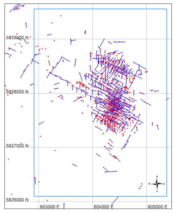
Figure 14-1 Drillhole Location Map Within the Block Model Limits Area (light blue) – All Drillhole Traces in Blue.
