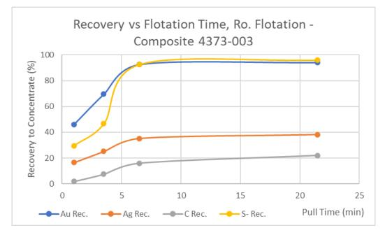
Figure 13-6 Kinetic Rougher Flotation Composite 4373-003, 80%-180µm Feed Size
