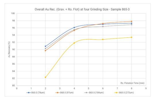
Figure 13-4 Sensitivity of Rougher Flotation to Grind Size
