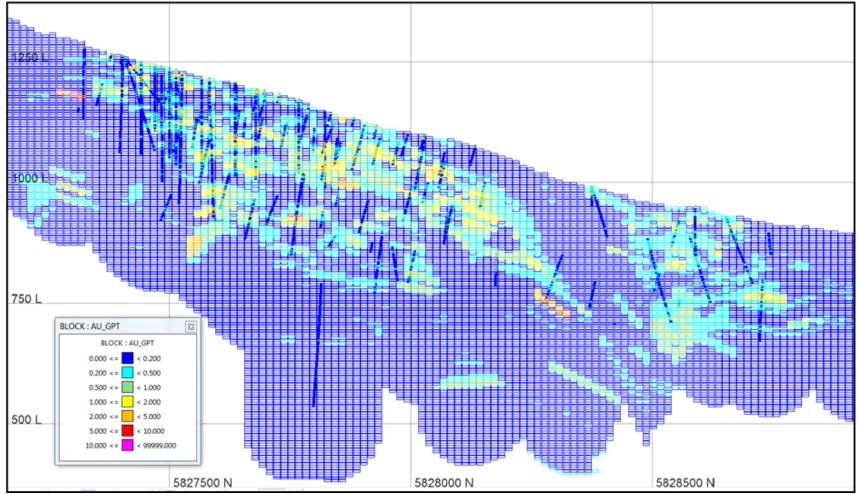
Figure 14-11 Gold Block Grade Estimates and Drillhole Grades – Section 604325E
