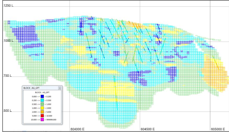
Figure 14-15 Silver Block Grade Estimates and Drillhole Grades – Section 5827800N
