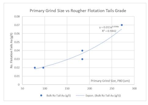
Figure 13-3 Primary grind size vs rougher flotation tailings grade
