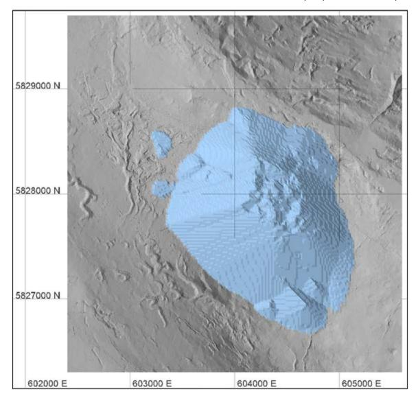
Figure 14-21 Mineral Resource Constraining Open Pit Shell – Plan View
