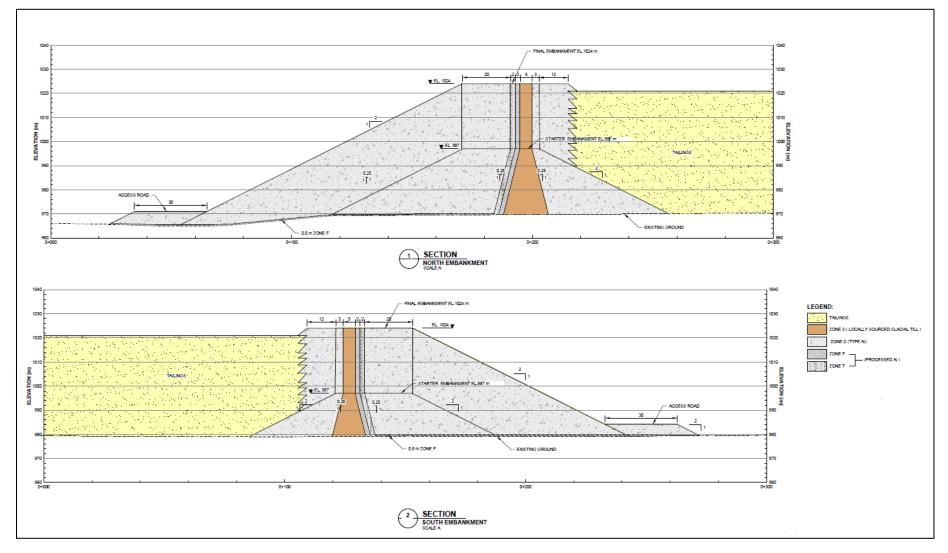
Figure 18-3 Cross sections of the TSF North and South Embankments
