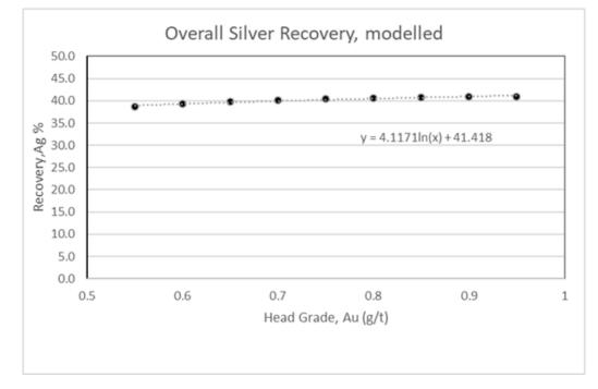
Figure 13-19 Overall Silver Recovery as a Function of Head Grade
