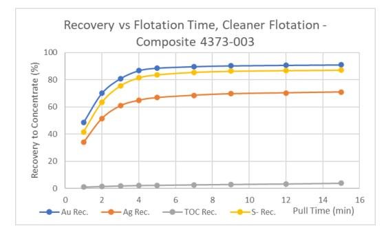
Figure 13-8 Kinetic Cleaner Flotation Composite 4373-003, 80%-180µm Feed Size
