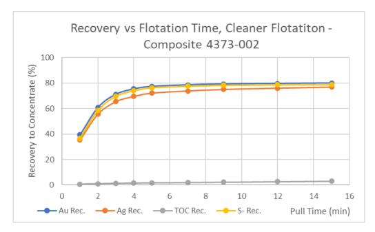
Figure 13-7 Kinetic Cleaner Flotation Composite 4373-002, 80%-180µm Feed Size
