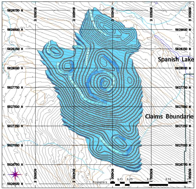
The General Arrangement, Figure 1-4 shows the mine layout for the pit, stockpiles, and haul roads.
