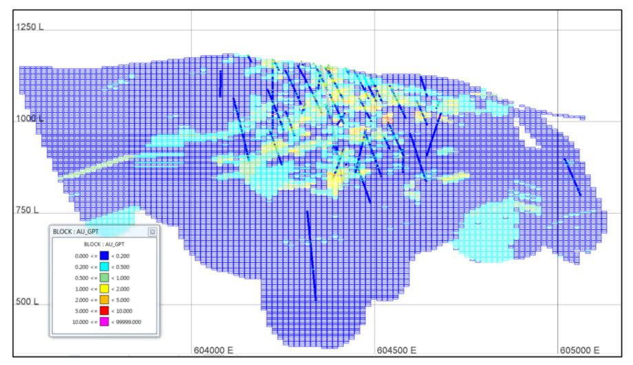
Figure 14-12 Gold Block Grade Estimates and Drillhole Grades – Section 5827800N
