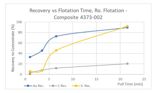
Figure 13-5 Kinetic Rougher Composite 4373-002, 80%- 180µm Feed Size
