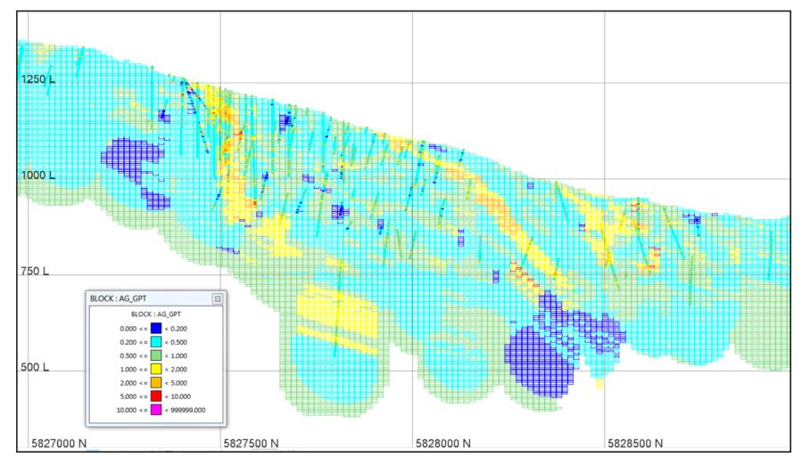
Figure 14-14 Silver Block Grade Estimates and Drillhole Grades – Section 604325E
