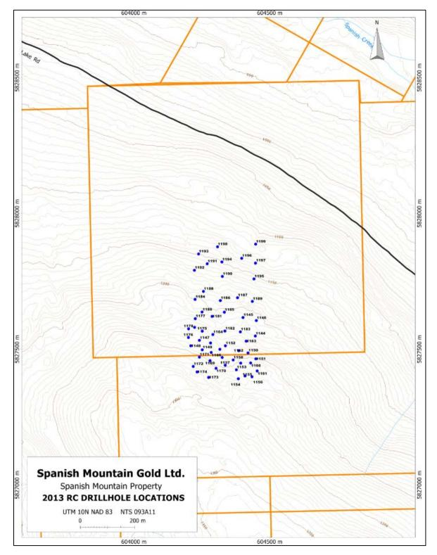
Figure 10-10 2013 Drillhole Locations
