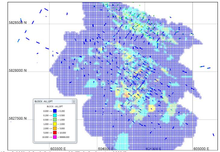
Figure 14-10 Gold Block Grade Estimates and Drillhole Grades – Level 925 El
